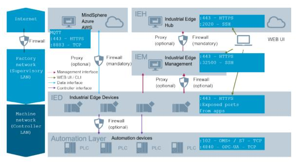
The customer IT security concept needs to decide and adjust the setup and network protection concept. The Industrial Edge Management and Edge Devices must not be operated in zero trust networks.
